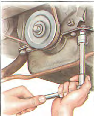
Tighten all the sump bolts evenly.
