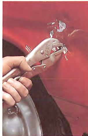
Small dents can often be pulled out more easily, depending on their location. Drill a small hole in the centre of the dent and screw a self-tapping screw in, but leave the head and a few threads exposed. Grip the head with self-locking grips and pull outwards.
