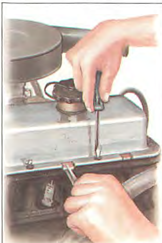
A rocker-cover gasket located by small tongues in the cover flange – position them properly before tightening down the cover.
