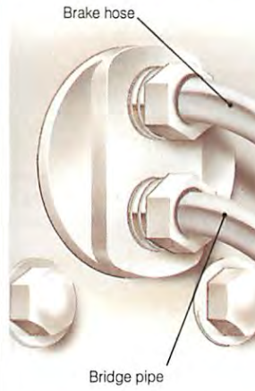
On a two-leading-shoe brake, disconnect the bridge pipe at the cylinder to be removed.
