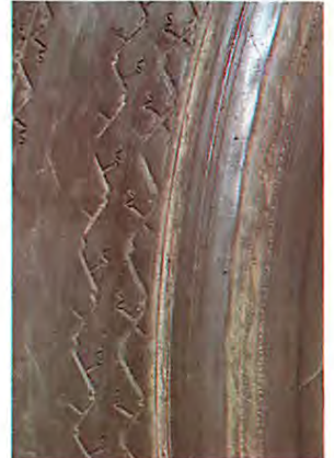
Fitting too wide a tyre may cause bodywork interference.
