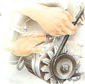
Loosen the pivot bolts on the generator, then on the adjuster strap.
