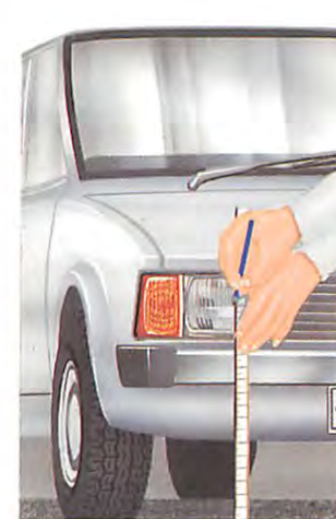
Draw two outer lines equidistant from the centre line and the same distance apart as the headlamp centres.
