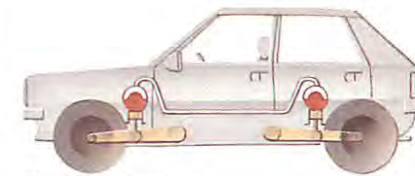
Hydraulic suspension Hydraulic suspension combines rubber springs with a damper system linking the front and rear wheel on the same side of the car.
