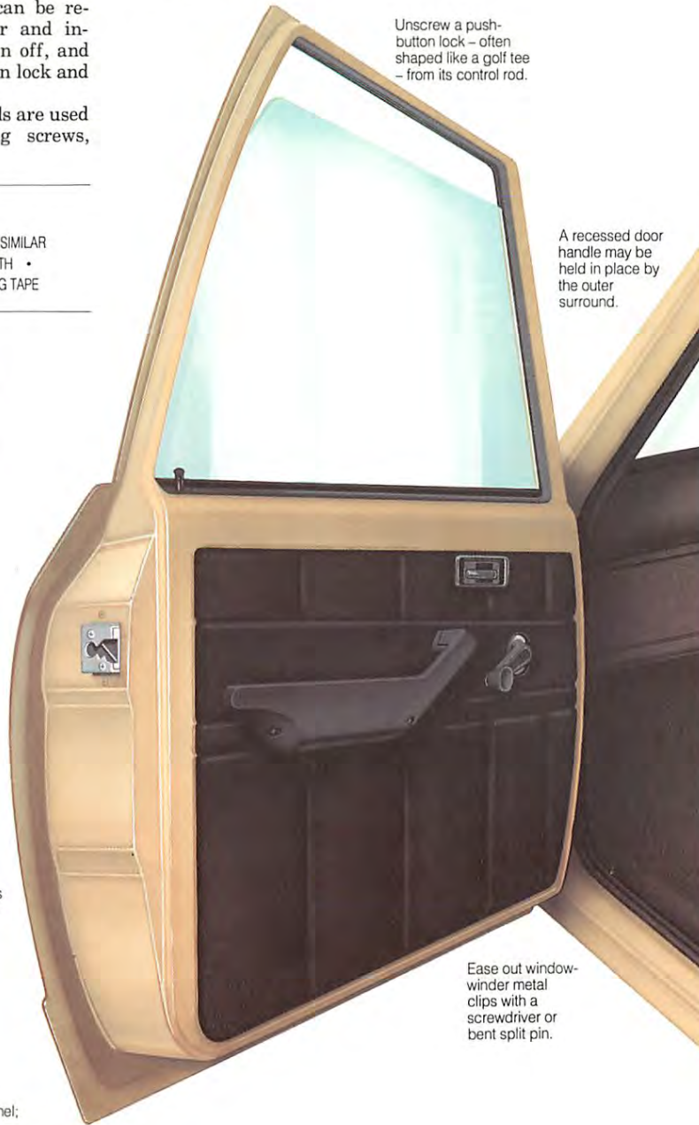
Arm-rest screws – usually cross-headed – are sometimes concealed underneath.
