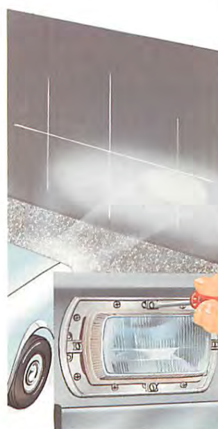
Use the top adjuster to lower the spot 2 in. (50 mm) below the cross. Cover the lamp and align the other in the same way.
