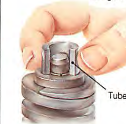
A short length of tube split lengthways to make a gap.
