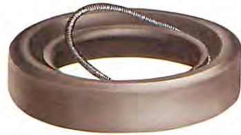
The dynamic seal surrounds a turning shaft. The lip always faces the oil it seals in, and the garter spring provides gentle pressure.
