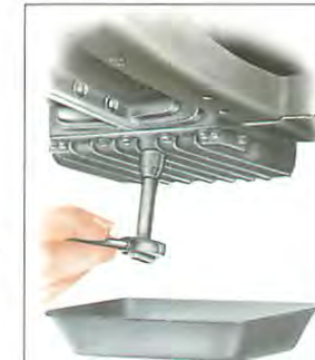
An automatic transmission that requires regular draining and refilling should be drained with the unit at running temperature. Remove the drain plug carefully, keeping hands and arms clear of the hot fluid, which can burn.
