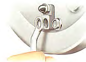
Two-bolt fixing method – remove both.
