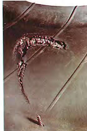
Tyre penetration by a screw can cause irreparable damage.
