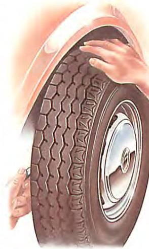
As you adjust, spin the wheel until it locks, then readjust gradually until the wheel rotates freely.
