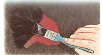
Apply brush-on underbody sealant thickly, working it into crevices.
