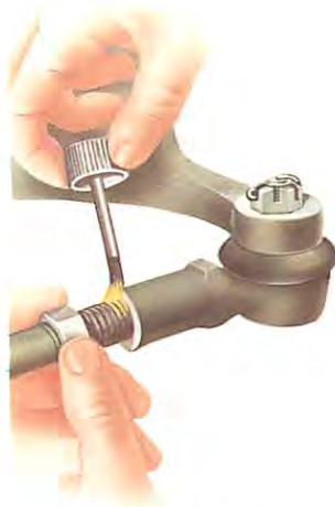
When the locknut is freed, mark the end of the ball-joint body and thread with a dab of brightly coloured paint as a guide when replacing.
