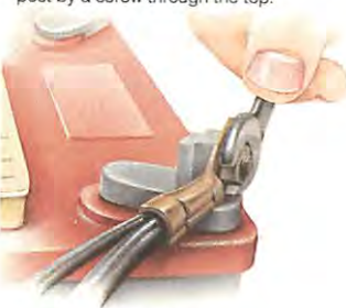
Unscrew the nut and bolt of a Ford-type connector.
