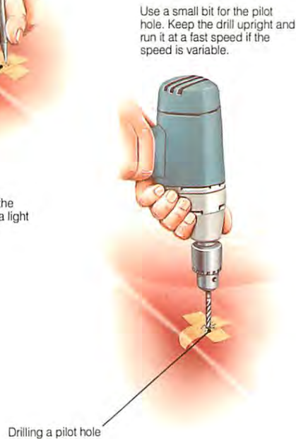
Drilling a pilot hole
