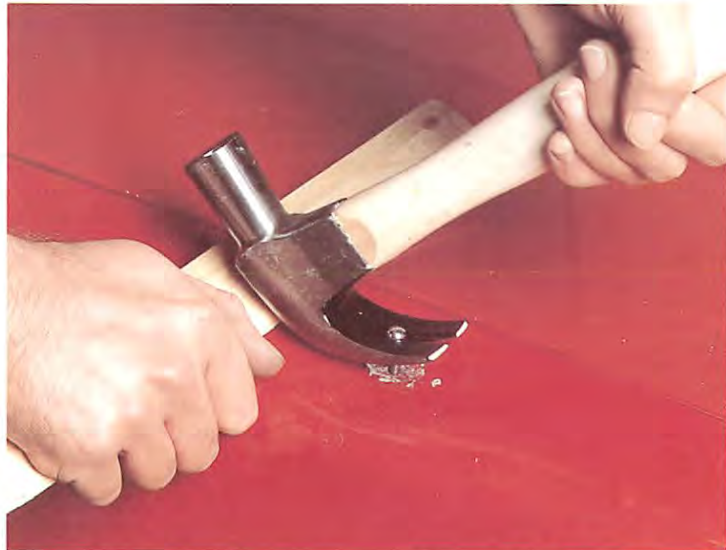
To pull out a large dent, screw a self-tapping screw in the centre and use a claw hammer
