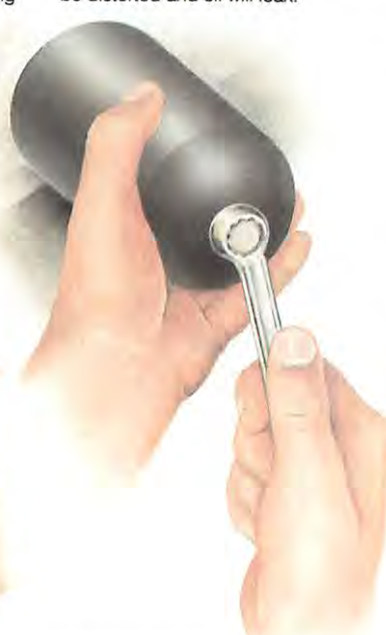
Tighten the central bolt until the sealing ring is compressed. Do not overtighten - this will ruin the sealing ring, causing a leak.
