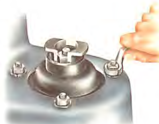
MacPherson-strut upper mountings have bearings on rubber blocks. Check the fixing plate nuts for tightness.
