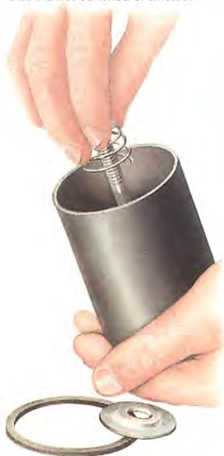
Fit the sealing ring in the mounting flange. Replace the spring over the central bolt, followed by the locating plate.
