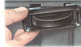
Sliding out a door-handle surround.
