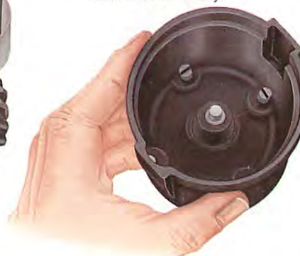
Before refitting the cap, check whether it is marked or cracked. If it is, renew it.
