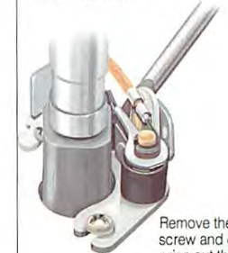
Slacken the terminal nuts and lift the lead.
