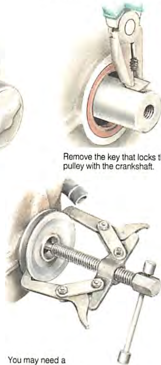
You may need a universal puller to remove the pulley.
