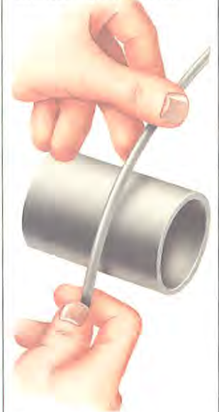
Tight bends should be made round a tube at least 2 in. (50 mm) in diameter.
