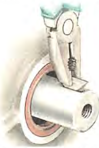
Remove the key that locks the pulley with the crankshaft.
