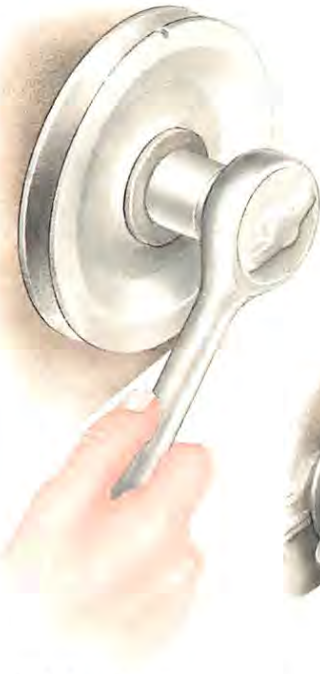
Jam the flywheel ring gear to prevent the engine turning while you undo the crankshaft pulley bolt.
