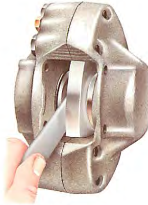
A strong but careful pressure is needed to lever the piston back.
