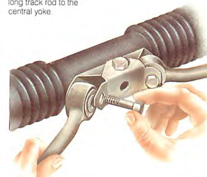
Screw up to the measured distance and tighten the locknut on a short track rod.
