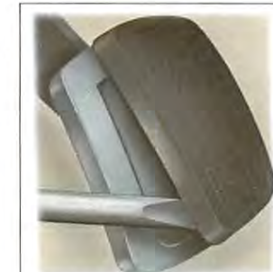
Use a screwdriver if necessary to remove or to fit a pedal pad.
