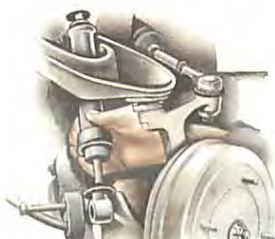
Push the damper rod in and lower it from the car.
