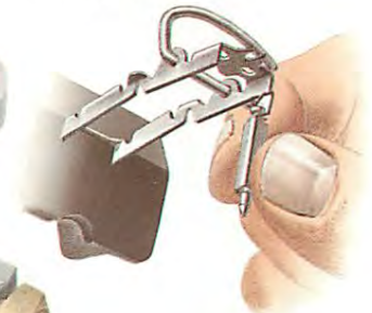
Lift the needle off the float to check it.
