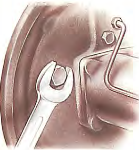
Turn the hexagonal bolts on the backplate to back the shoes off the drum.
