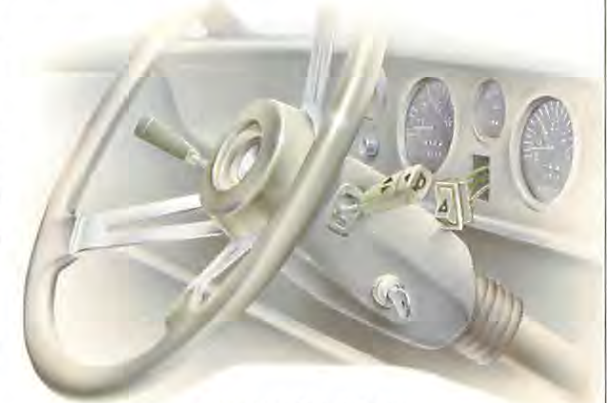
A hazard-warning switch can often be pulled out for testing.
