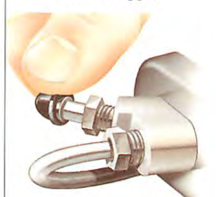
Sometimes the bleed nipple must be removed before the brake pipe can be pulled through. Save its small cap.
