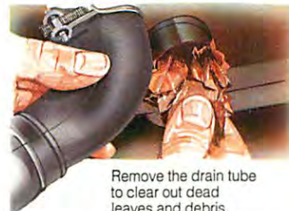
Test the drain valve with a forefinger.
