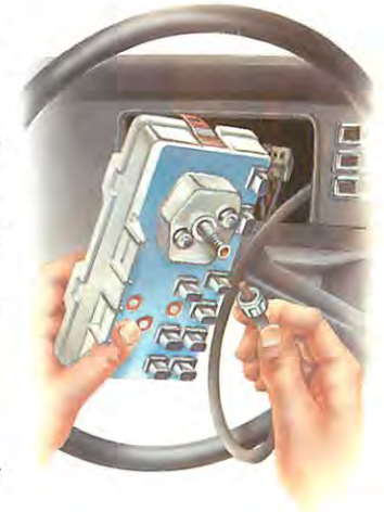
Disconnect the cable from the speedometer and check for loose fixings and worn drive ends.
