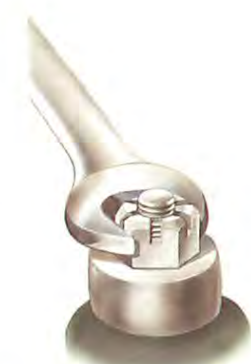
Slacken the nut a few turns but do not remove it, so that the upper arm of the separating tool can bear against it.
