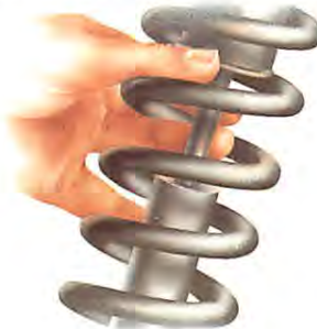
Dampers are fitted inside the springs of a coil-spring suspension system.
