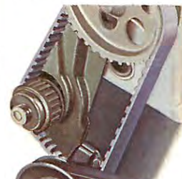
The water pump on the VW Golf is driven by the camshaft drive belt.
