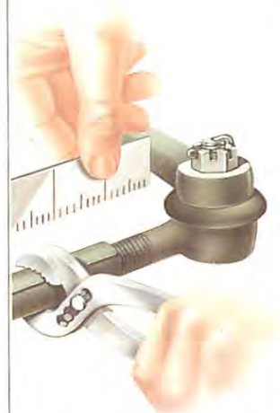
Use a ruler to measure accurately the length of thread showing on a ball joint that screws into the track rod.
