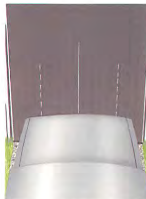
Draw two outer lines equidistant from the centre line and the same distance apart as the headlamp centres.
