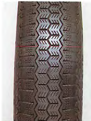
Shoulder wear – the tyre has been run at too low a pressure.
