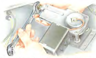
The rack tube is secured to the motor by a nut. Loosen it to free the tube.
