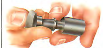
When pushing the cup seal into the cylinder, do not turn the lip under.
