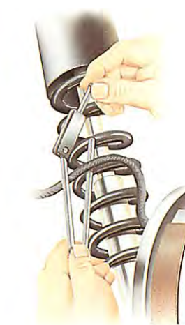
Seal off the flexible brake hose with a hose clamp.
