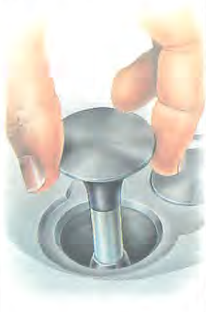
Check the valve stem and guide by trying to move the valve from side to side in the guide.
