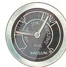
If the needle drifts between 5 and 19 there may be a leak at the cylinder-head gasket.
