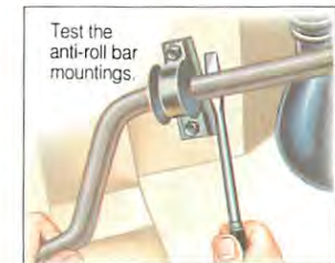
Check stabiliser arm joints for movement.
