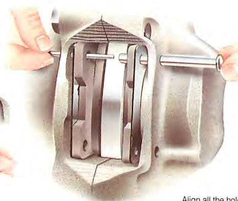
Replace anti-squeal shims with the arrow pointing in the direction of forward rotation.
