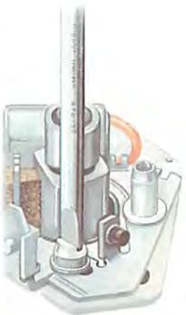
Undo the single fixing screw and remove the fixed contact plate.
