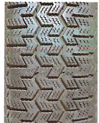
Feathering – wheel misalignment such as excessive toe-in or toe-out.
