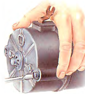
Remove the screws holding the endplate to the body.
