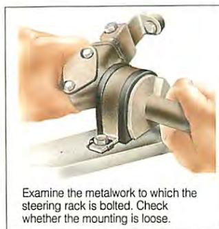
Clamps or brackets secure the steering rack to the front cross member or bulkhead.
