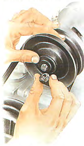
Replace the pulley front half with the shim on the outside of the pulley, between it and the nut or nuts.
