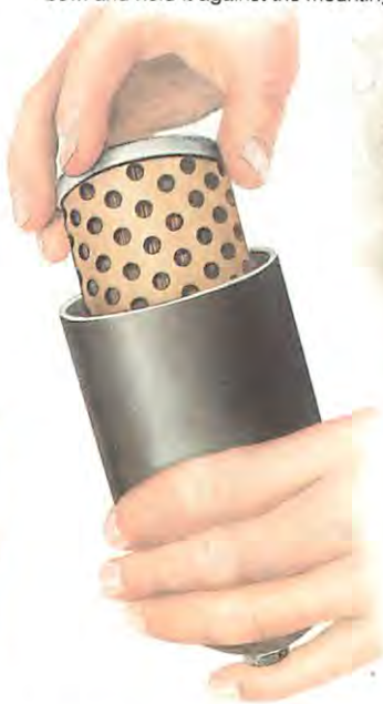
The new element fits over the central bolt, and the assembly is bolted to the mounting flange.
