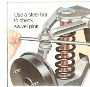
Lever joints sideways and look for movement.
