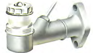
An aluminium-bodied centre-valve (CV) master cylinder (single-circuit type).
