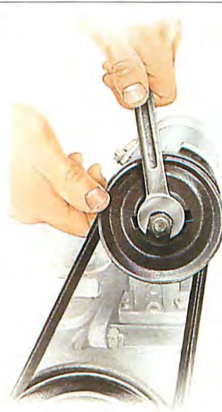
Unscrew the nut or nuts to split the two halves of the pulley.
