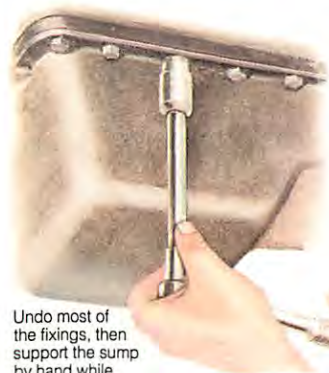
You may have to remove the cover to reach rear sump nuts.
