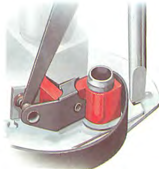
Set the gap with a screwdriver.
