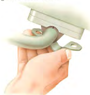
Remove washer clamps, spacers and other parts, keeping them in order.
