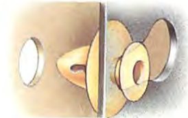
Plastic press studs are the commonest method of panel fixing.
