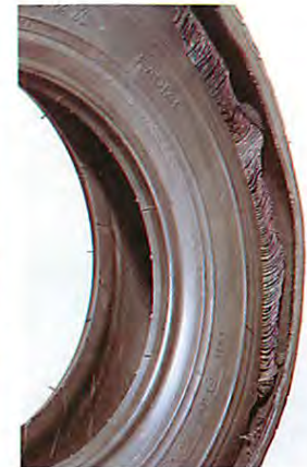
Running on a flat tyre will cause the carcass to break up.
