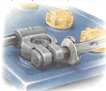
Loosening the bolt of a clamp connector.
