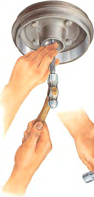
When the races are the same size, push out one with a punch or chisel, push out the other with a socket.
