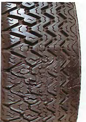
Rasped tread – constant fierce braking or faulty brakes.
