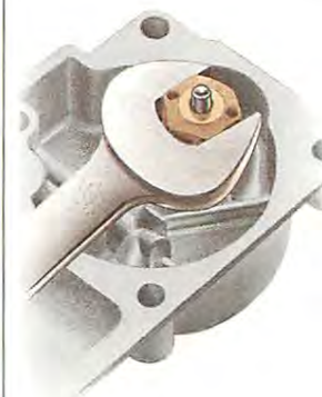
Some needle-valve assemblies are removed with a spanner.
