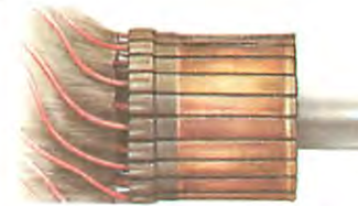
Glazing The commutator segments have a varnished look. This coating may be due to dust and water inside the casing, or to particles worn from the brushes or the mica insulation strips between segments.
