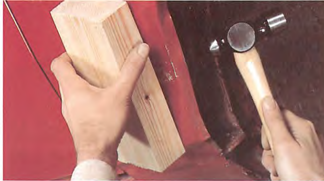
Hold a flat piece of wood over the outside of the dent. Use the rounded end of a ball-
