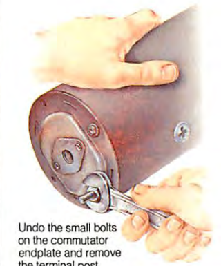
Unscrew the two slot-headed bolts in the endplate.
