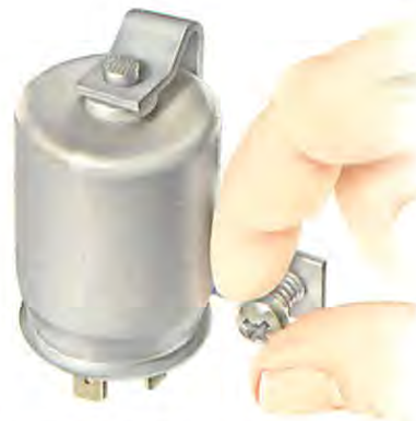
Label the leads when changing this type of unit, to avoid confusing them.
