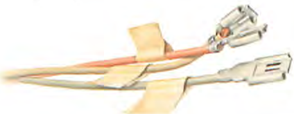
Label the leads when changing this type of unit, to avoid confusing them.
