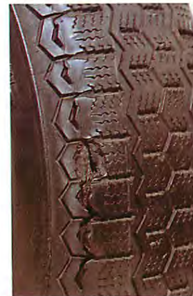
Tread separation may be due to age or oil contamination.
