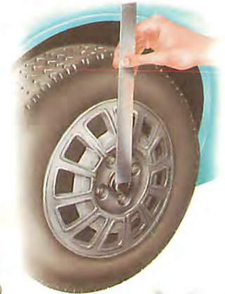
Measuring the ride height of the car will reveal a drop in the suspension.
