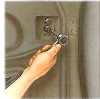
On some cars you can reach the bolts on the door side of the hinge with a socket and bar, after removing all or part of the trim.
