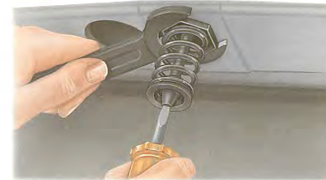
Loosen the locknut and adjust the dovetail lock for length.
