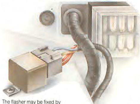
The flasher may be fixed by means of screws.
