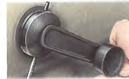
Push out fixing pin with a knitting needle.
