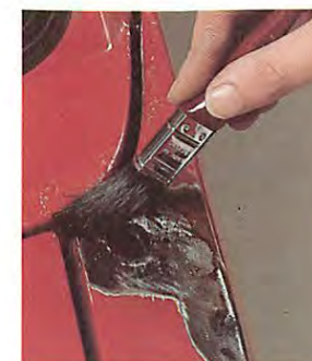
Apply rust-removing fluid with a paint brush – do not let it splash on to good paint. If it does, wipe off immediately.
