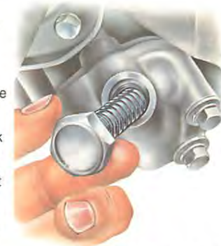
Unscrew the plug and remove the valve spring and the plunger or ball.
