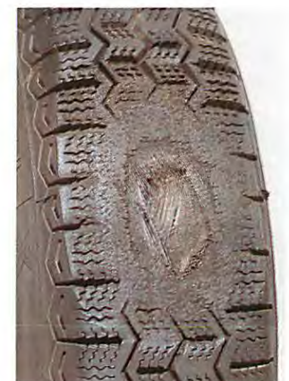
Brake flat (exposed cords due to locked-wheel braking at high speeds).
