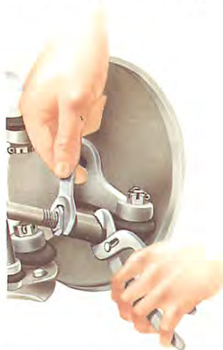
Grip the 'flats' on the ball-joint body to hold it in exactly the same position while you loosen the locknut with a spanner.
