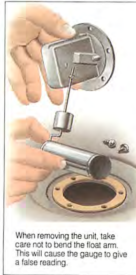
Petrol tank The tank may be fitted in the boot under the trim, with a top-fitted sender that incorporates the fuel pipes.
