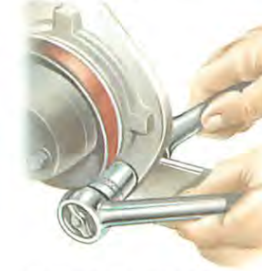
Slacken the pivot bolt or bolts slightly, but do not remove.
