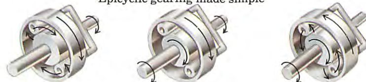
With central sun gear locked, planets turn round it; carrier and outer ring turn same way.
