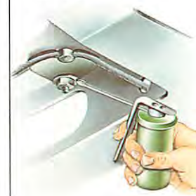
On a Mini, the cable is held in a sector on the rear radius arm. Keep the sector pivot oiled to prevent it seizing.
