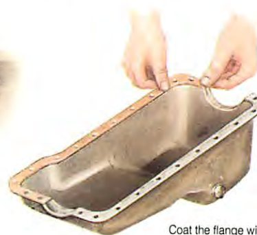
Coat the flange with gasket sealant, then carefully fit the flat parts of the gasket.
