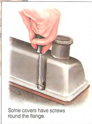
Lift off the cover. It may need a gentle sideways tap to free it.
