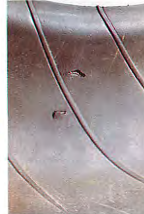
Striking a kerb could have caused this internal rupture.
