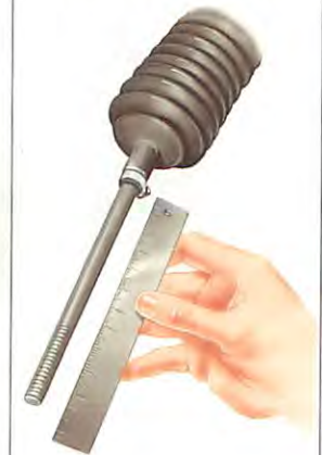
Measure or mark the position of the end of the gaiter.
