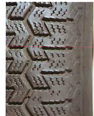
Shoulder wear – constant hard cornering at high speeds.
