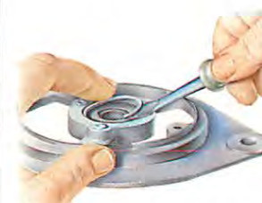
Take out the wire circlip with a small screwdriver.
