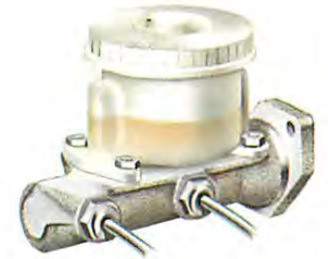
A cast-iron compression-barrel (CB) master cylinder (dual-circuit type).
