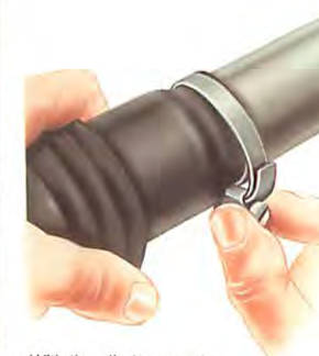
With the clip loosened, slide back the gaiter.
