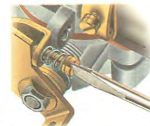
The throttle-stop screw increases engine speed when turned clockwise.
