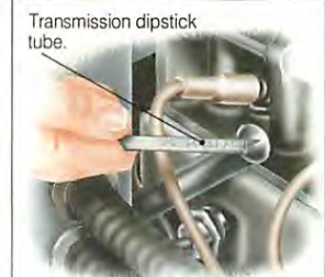
Clean around the dipstick area to avoid dirt getting into the transmission.
