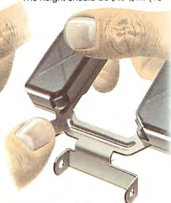
Bend the tag to adjust the float height.
