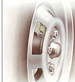
Look through the hole in the wheel rim to check pad thickness.
