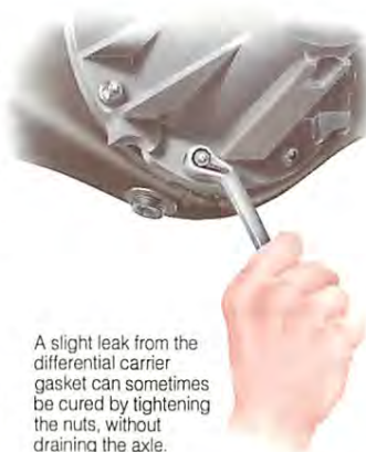
The filler plug may have a hexagonal head, or a square hole that takes a socket drive.
