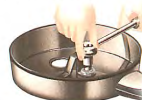
Loosen the securing bolt in the centre of the cleaner housing.
