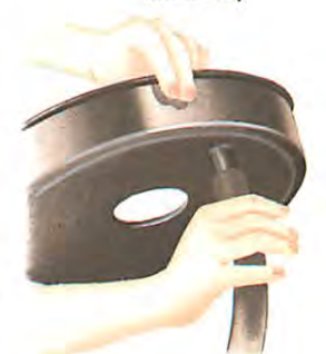
Remove crankcase breather hose from underneath the air cleaner.
