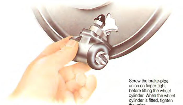
Check that the belled end of the brake pipe is clean and undamaged.
