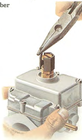
Pull the adjuster stop straight off.
