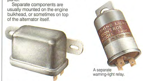
A typical separate type of electronic regulator.
