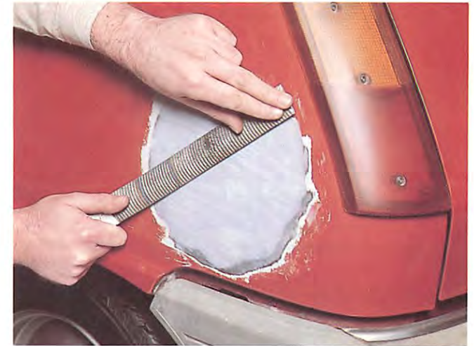
Roughly shape the hardened surface with a rasp, then change to a hard rubber
