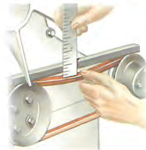
Pull the belt hard away from a straight-edge to measure deflection.
