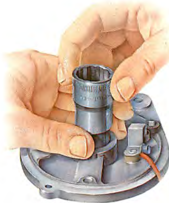
Select a socket the same diameter as the bush.
