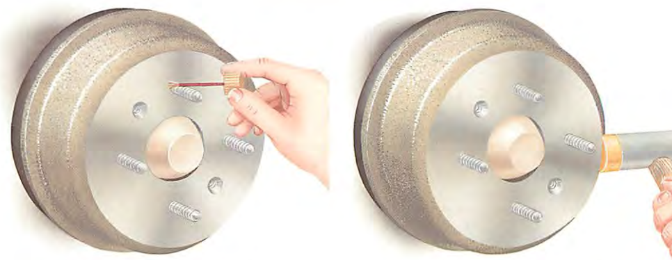
If the drum sticks, tap round the edge with a soft-faced hammer. Take care not to hit the lip of the drum or the backplate.
