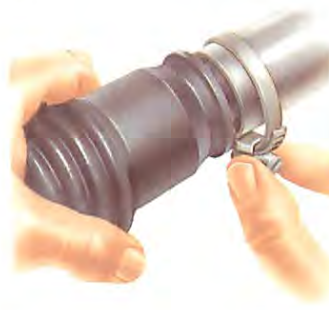
Ease the gaiter into place on the rack housing.
