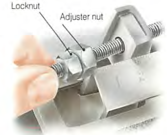
Measure between the adjuster nut and lever, and compare with the maker's specification. Adjust as necessary.
