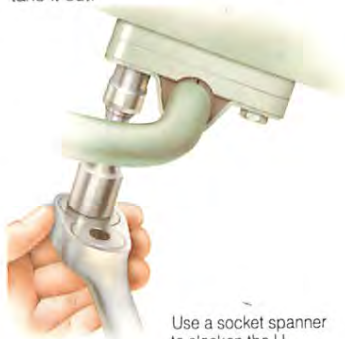
Use a socket spanner to slacken the U-clamp mounting bolts and nuts.
