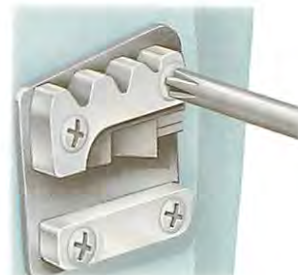
Loosen the locknut and adjust the dovetail lock for length.
