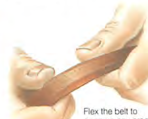
Flex the belt to open up any cracks. Replace a worn belt as soon as possible.
