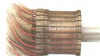
Scores and pits Usually pitting and scoring of the commutator segments are caused by electrical arcing between the commutator and badly fitted, poorly seating or worn-out brushes.
