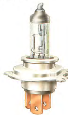
A halogen headlamp uses more power, but gives more than twice the illumination.
