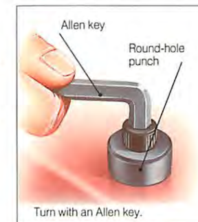
Enlarge the pilot hole.
