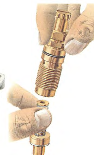
With the holder removed, pull out the jet.
