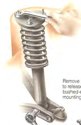
Undo the spring-cup mounting nuts under the bonnet.
