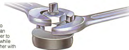
Where there is one securing nut, hold the flat or squared end of the pin with self-locking grips while you undo the nut with a spanner.
