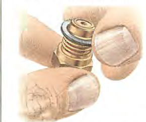
Sometimes you add a washer to the needle valve to adjust the float level.
