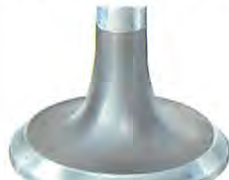
The valve head should have a small step between the face and the seat. A knife-edged valve should be replaced.
