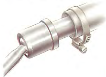
Hang the clip on the rack housing.
