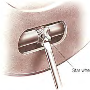
Use a large screwdriver to turn the star wheel.
