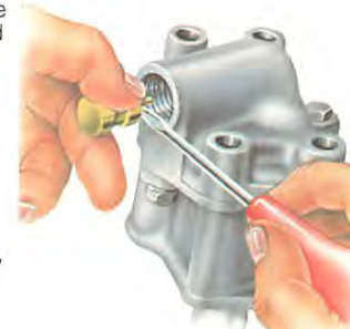
Release a stuck ball or plunger by gently prodding with a thin screwdriver.
