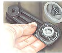
Slide a metal clip back out of its slot.
