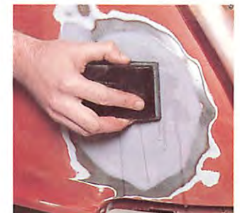
Use progressively finer grades of wet-and-dry paper to get a smooth finish.
