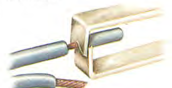
Remove insulation with a wire stripper.
