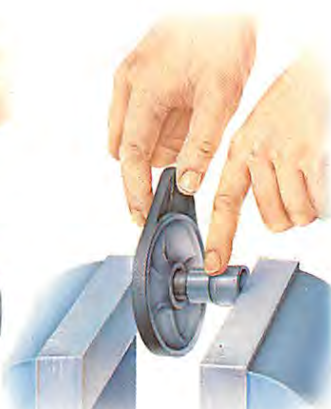
Press the new bush in with a vice, making sure it is aligned in the housing.
