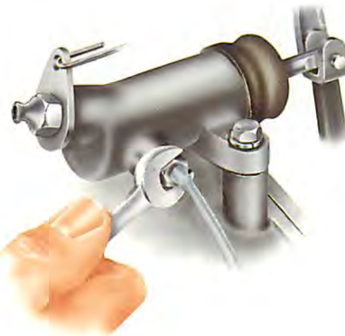
Loosen the pipe union nut on the side of the cylinder and undo the release-arm return spring. Remove the clevis pin from the release arm.
