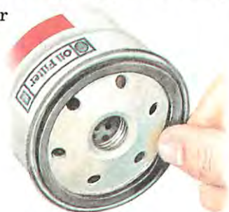
Smear the outer face of the sealing ring with clean engine oil.
