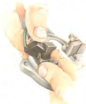
Push the spring to one side and remove the brush.
