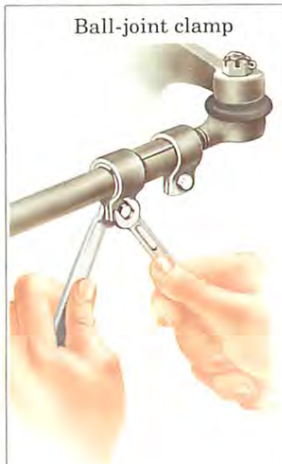
Loosening the clamp which secures some ball joints. Both clamp bolts must be slackened to free the joint.
