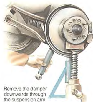
Push the damper rod in and lower it from the car.
