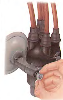
If the distributor has a vernier timing control, set it midway between advance and retard. Turn the knob fully anti-clockwise, then fully clockwise counting the number of turns. Divide the number by two to find the midway position.
