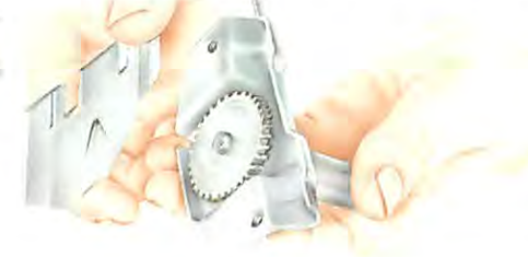
Remove the two screws holding the wheelbox together. Pack the box with high-melting-point grease.
