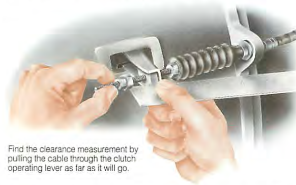
Measure between the adjuster nut and lever, and compare with the maker's specification. Adjust as necessary.
