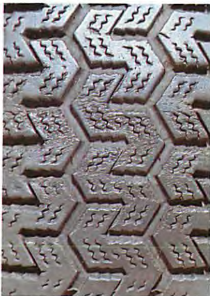
Ridging wear – caused by friction and heat from harsh motoring.
