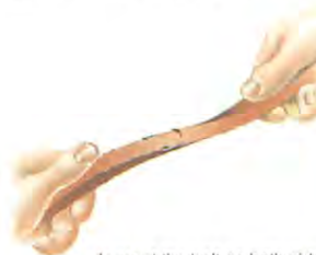
Inspect the belt on both sides for nicks, cuts, fraying and score marks.
