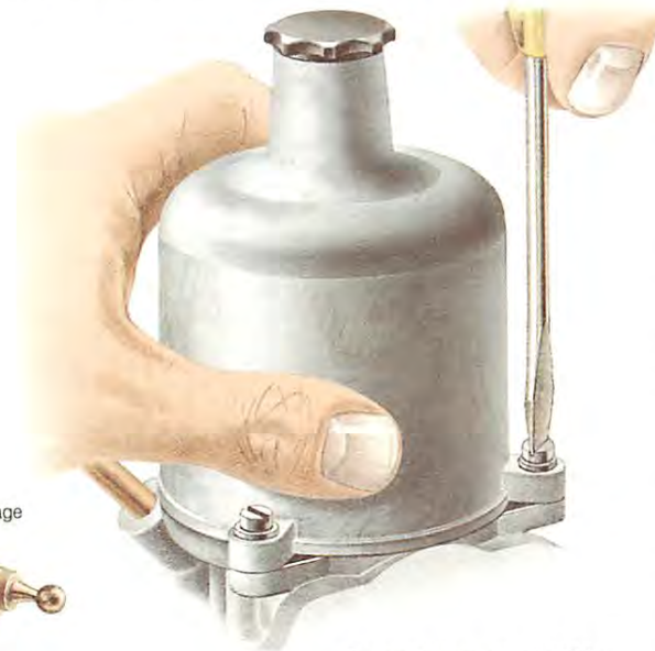
Remove the screws to take off the dashpot. Before lifting it off mark the dashpot and flange.
