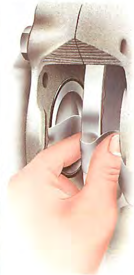
Clean the outer edges of the disc by pinching it with emery cloth.
