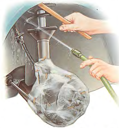
Use a powerful jet of water. Spray in corners until water runs clean.
