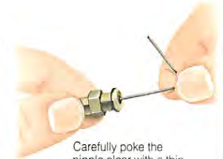
Carefully poke the nipple clear with a thin wire.
