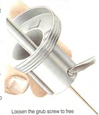
Lift out the piston and jet-needle assembly, taking care not to bend the needle.
