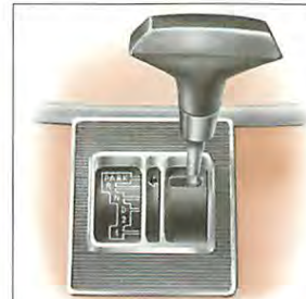
Let the engine run for two minutes with the selector at park 'P'.
