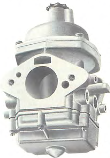
The CD3 is a fixed-jet carburettor and you need a special tool to reset the mixture control, which is done by altering the height of the jet needle.
