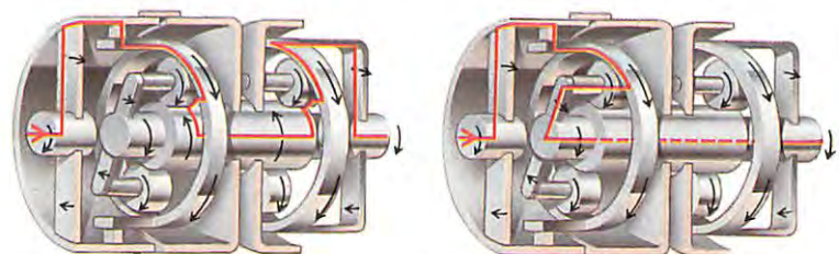
Drive one (first gear) The forward-drive clutch is engaged and the engine turns the first ring gear.
