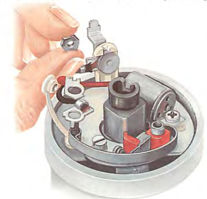
Remove the nut from the threaded top of the terminal post, and take off the connections.
