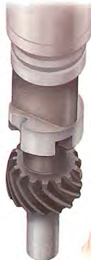
Some distributors have a skew-gear drive fitting.
