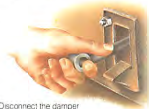
Disconnect the damper arm from the suspension. Move the arm slowly up and down.
