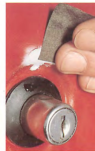
When the stopper has hardened, flatten it down with medium and fine grades of wet-and-dry, used wet.
