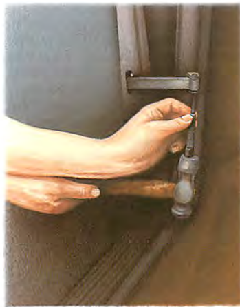
A door check strap (restrainer) is often held with a pivot pin. Release the strap by tapping out the pin with a hammer and punch.
