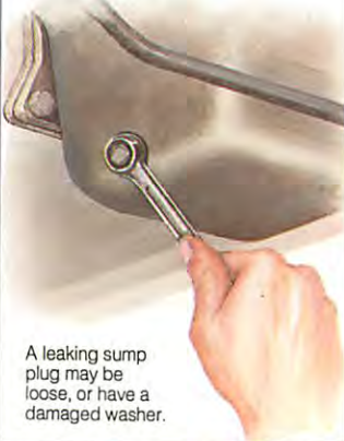
Tighten all the sump bolts evenly.
