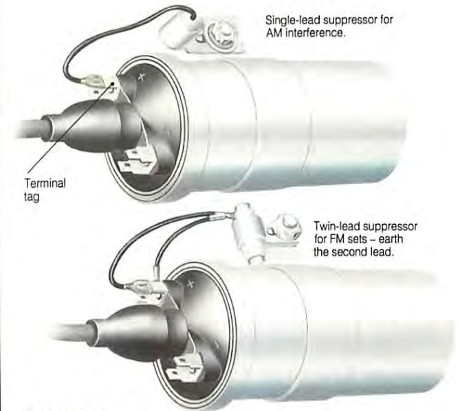
Two types of coil suppressor for AM or FM radio reception.
