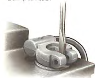
Loosening the bolt of a clamp connector.
