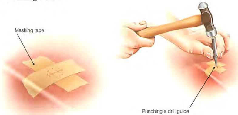
Punching a drill guide
