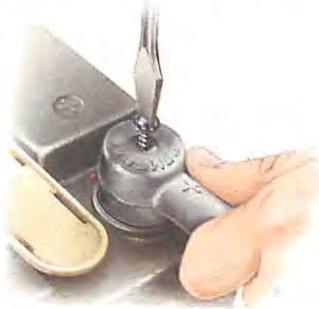
A cup connector secured to the terminal post by a screw through the top.
