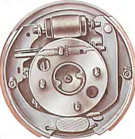
The brake drum can then be removed to reveal the shoes and automatic adjustment mechanism.
