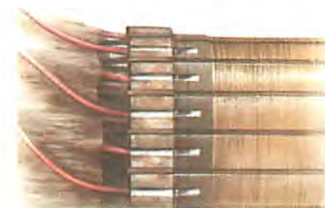
Melted solder Overheating can melt the solder connections between the segments and the armature windings. Severe cases show as a ring of melted solder around the inside of the casing.
