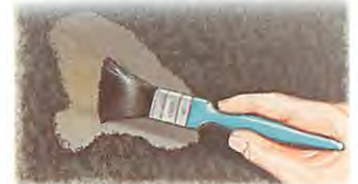
Use anti-rust preparation on bare metal and follow maker's instructions.
