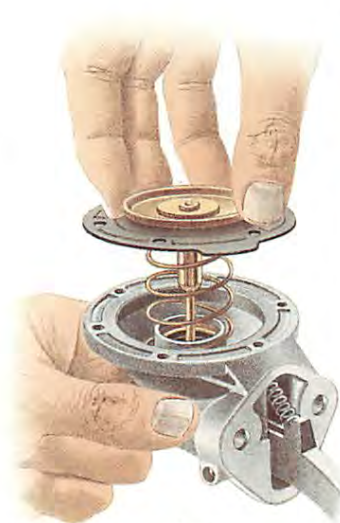
On AC-Delco pumps, give the diaphragm a quarter turn to release the T-shaped end of its link from the slot in the lever.
