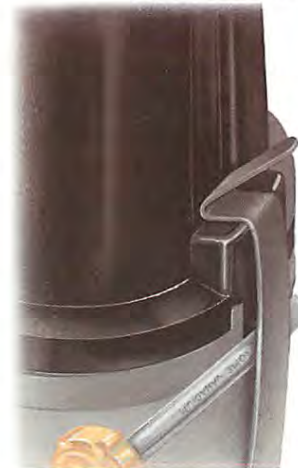
The distributor cap is usually held on by spring clips.
