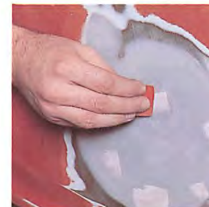
Fill small dents and scratches with stopper, and lightly rub down.
