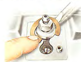
The E-clip fits on concave side first.
