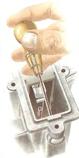
Push out the blanking disc with a screwdriver.
