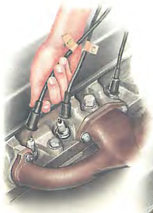
Remove the plug leads by gripping the caps, not by pulling on the leads which may damage them. Label the leads if necessary to avoid confusion when refitting them.
