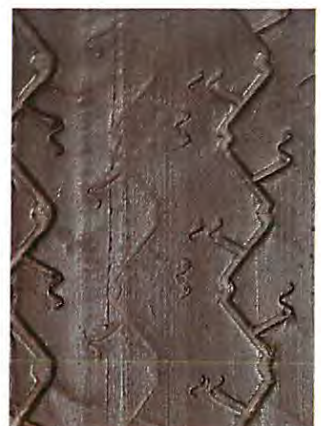
Brake flat (heavy braking will eventually cause a bare patch).
