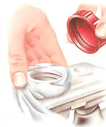
Wrap some rag around the mouth of the reservoir to absorb any brake fluid that may overflow.
