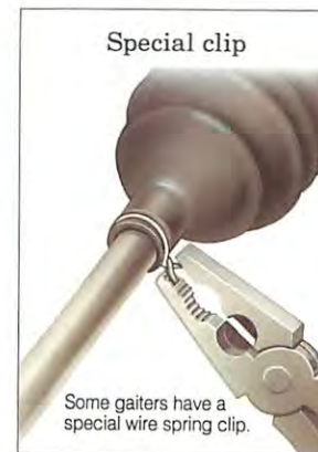
With the clip loosened, slide back the gaiter.
