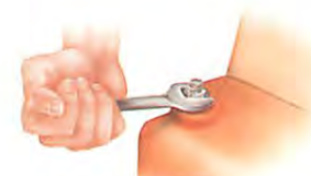
The top of a turret mounting is usually on the wheel arch inside the boot. Test it for tightness.
