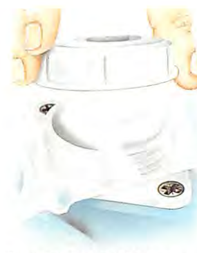
Screw down the reservoir cap over a sheet of thin plastic.
