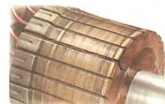
Faulty insulation The mica strips stick up between segments, stopping the brushes making contact. This is caused by wear or arcing removing surface copper. One of the segments has also cracked.
