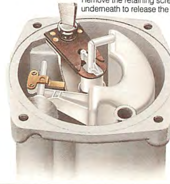
Remove the retaining screw from underneath to release the jet.
