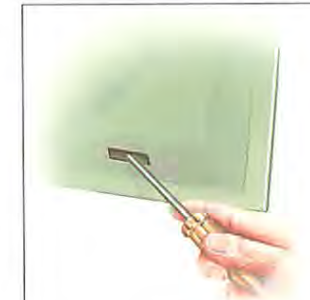
Use a thin-bladed screwdriver to poke out dirt blocking drain holes in the bottoms of doors.
