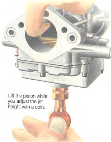
Turn until the jet height is just above the bridge in the carburettor bore.
