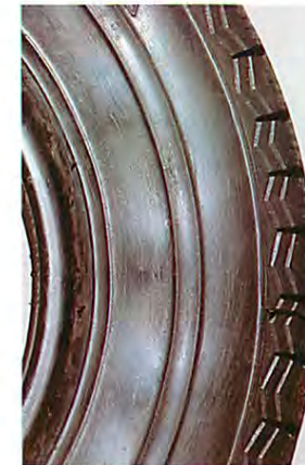
Fuel or oil on a sidewall will eventually weaken the tyre.
