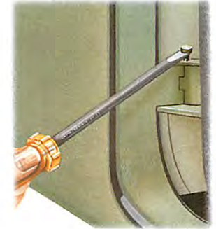
Solid pins with projecting heads can often be levered out with a screwdriver inserted under the head of the pin.
