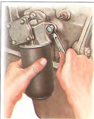
Tightening the pump adaptor bolts may cure a slight leak from the mounting flange.
