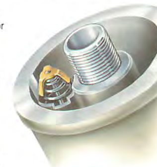
Some types of oil-pressure relief valve cannot be removed.
