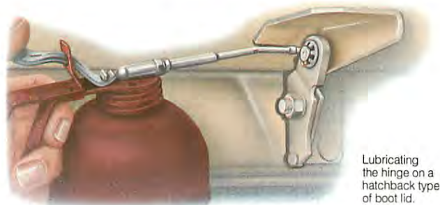
Lubricate the restrainer with clean engine oil.
