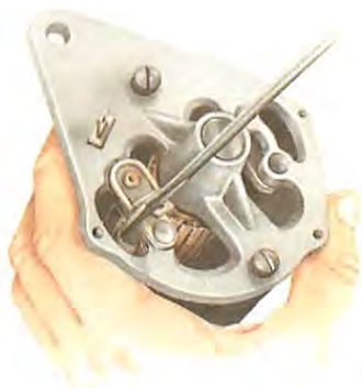
Use a screwdriver through the hole in the endplate to move the end of the coiled spring from the side to the top of the brush, to push it into contact with the commutator.
