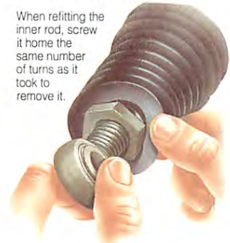
Set the eye vertical, then screw up the locknut.
