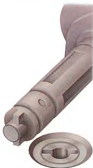
The distributor driving gear may be an offset dog – a tongue that fits into a slot.
