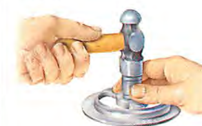
Tap the bearing out, using a socket as a drift.
