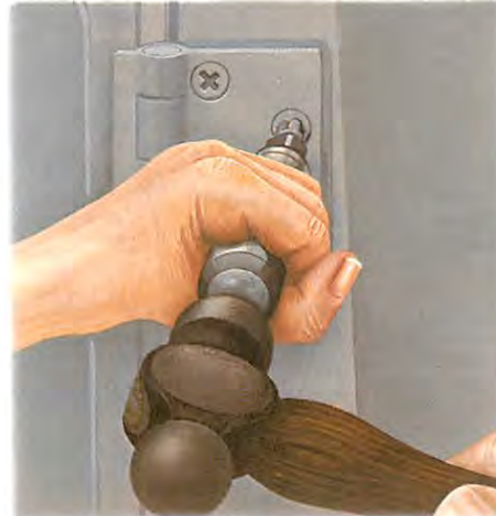
To undo cross-slot hinge bolts you may need to use an impact screwdriver.
