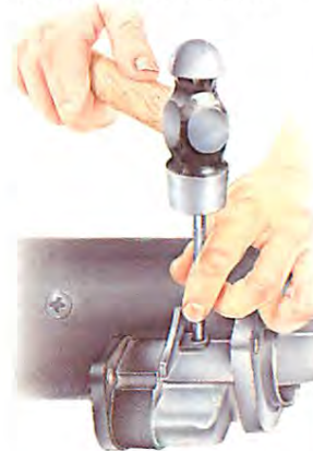
The pivot pin may be a force fit – if so, drive it out with a punch and hammer.
