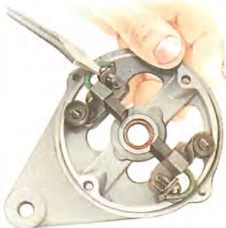
Undo the screws holding the brush cables.
