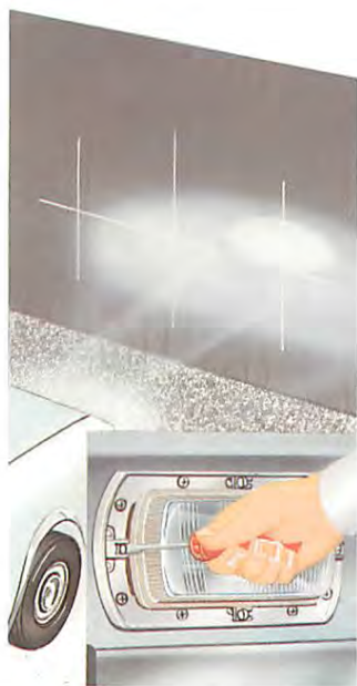
With one headlamp covered, turn the side adjuster(s) of the other to centre the bright spot on the vertical line.
