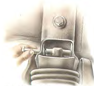
Note whether the bolt head on the top mounting fits towards the front of the car. Refit the same way.
