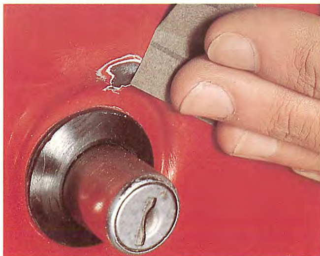
Clean up small chips in paintwork with a scrap of coarse wet-and-dry paper, used
