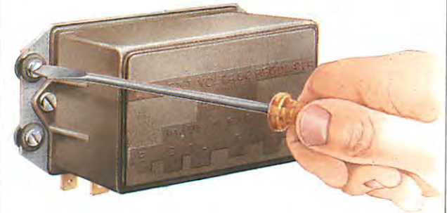
The control box is usually held by two or three screws – remove them.
