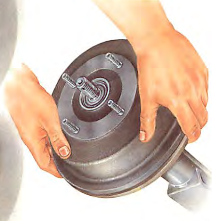
Replace the hub carefully, so as not to disturb the bearings or races.
