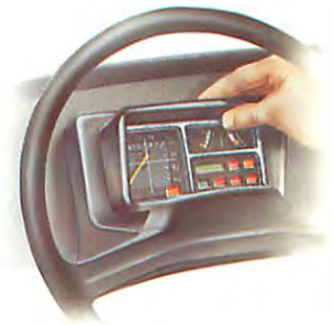
Gently prise the cowl off its clips with your hands or a screwdriver, then draw it out.
