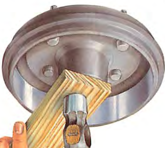
Tap new grease seals into place using a hammer, protecting the seal with a flat piece of wood.
