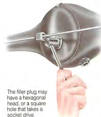
Use a large container to catch the dirty oil.
