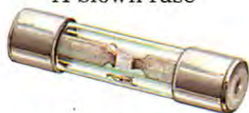
A fuse is 'blown' when the connector between its two ends melts under an overload of current.
