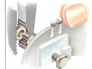
Slacken the terminal nuts and lift the lead.
