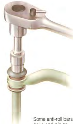
Some anti-roll bars have end-pin or eye-bolt fittings.
