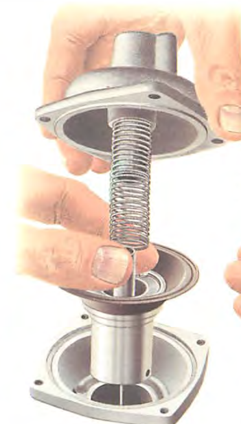
For larger adjustments, lift out the piston and spring.
