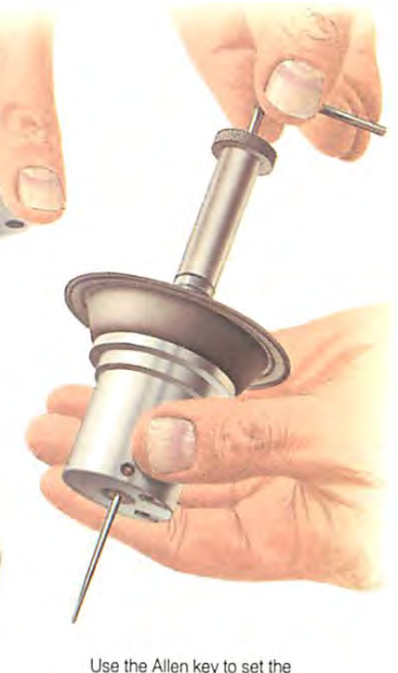
Use the Allen key to set the needle in a midway position.
