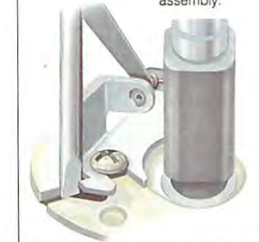
The gap is adjusted by swinging the assembly around the moving contact pivot point.
