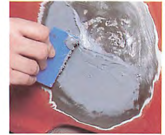
Once the surface has been prepared, mix up sufficient body filler and smooth over with the plastic spatula.
