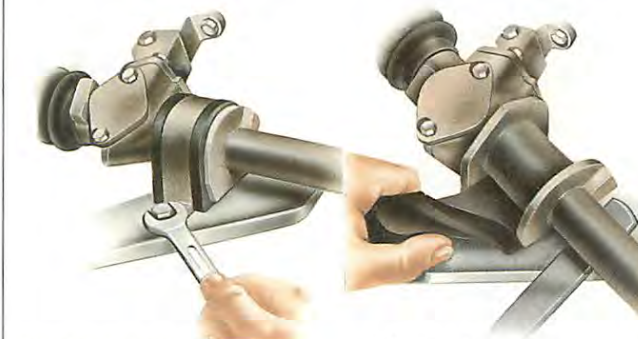
Working first on one bracket, then the other, unscrew the retaining bolts (and washers if fitted) and remove the bracket.
