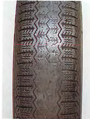
Centre tread wear – caused by over-inflation.
