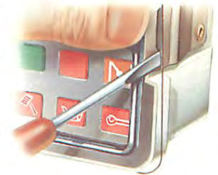
Use a thin screwdriver to ease the panel lip out of the clip that holds it at each side.
