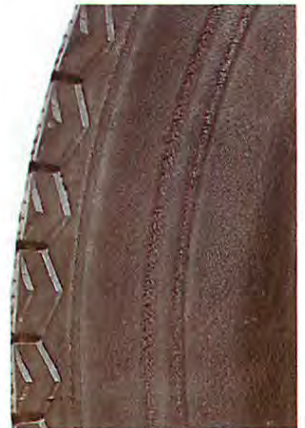
Ozone in sea air causes crazing of the sidewalls.
