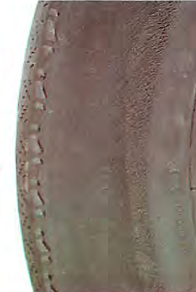
Kerbing will also damage and weaken the outer sidewall.
