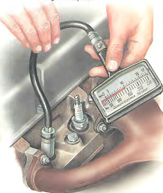
The compression tester usually screws in although some models have a rubber plug.
