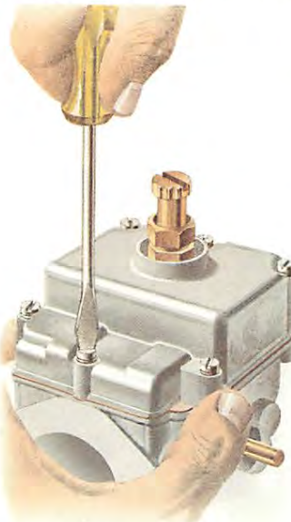
Remove the six float-chamber securing screws.
