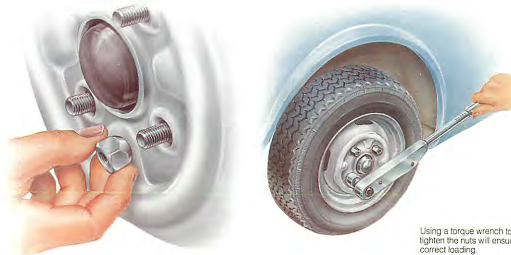
The conical faces of wheel nuts go into countersunk wheel holes.
