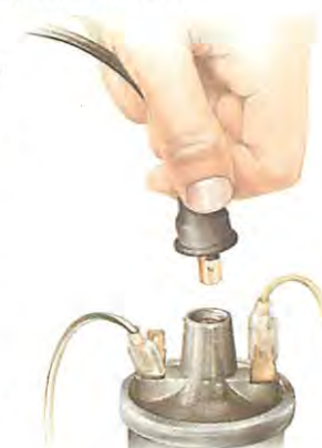
Remove the high-tension lead from the coil, so the engine will turn over but not start.
