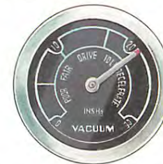
A zero reading at idling speed after a 22 reading at high speed indicates worn piston rings.
