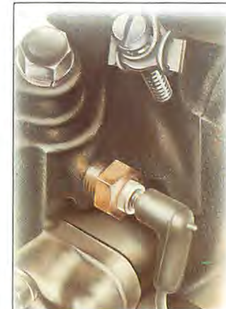
To remove a coolant-temperature sensor, first drain off the coolant to below the level of the sensor.
