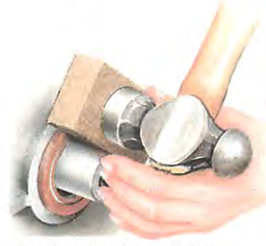
Tap in the new seal with a wooden block, keeping it absolutely straight.
