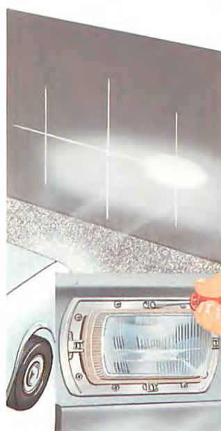
Turn the top adjuster of the headlamp until the bright spot is centred on the horizontal line as well.
