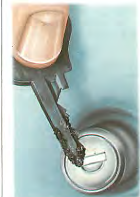
Use graphite powder on the key to lubricate a lock.
