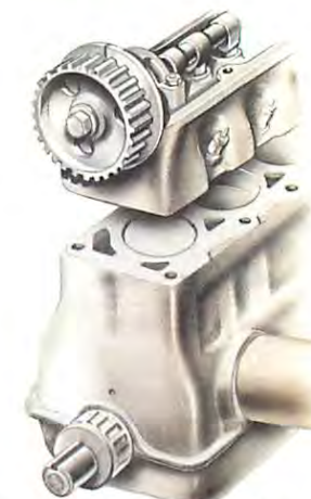
Before refitting the head to an OHC engine, set No. 1 cylinder to TDC and line up the corresponding marks on the camshaft drive-belt sprocket. A chain-drive sprocket has similar marks.
