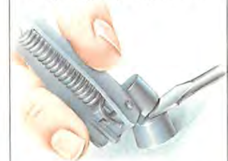
Some arms are held by a spring clip. To remove, lever the clip up and out.
