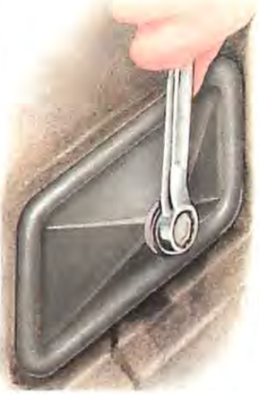
The side cover may be held by one or more bolts. Undo them, then prise it off carefully.
