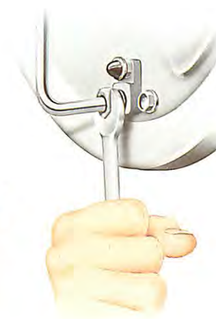
Loosen the union before freeing the wheel cylinder.
