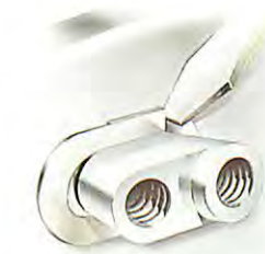
Slide off the clip by tapping each leg with a hammer and screwdriver.
