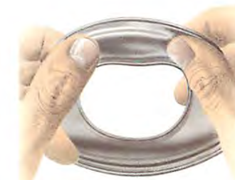
Pull the diaphragm gently and hold it up to the light to show up any pinholes.
